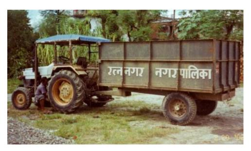
Tractor with Modified Trailer to Accommodate Large Amount of Waste
