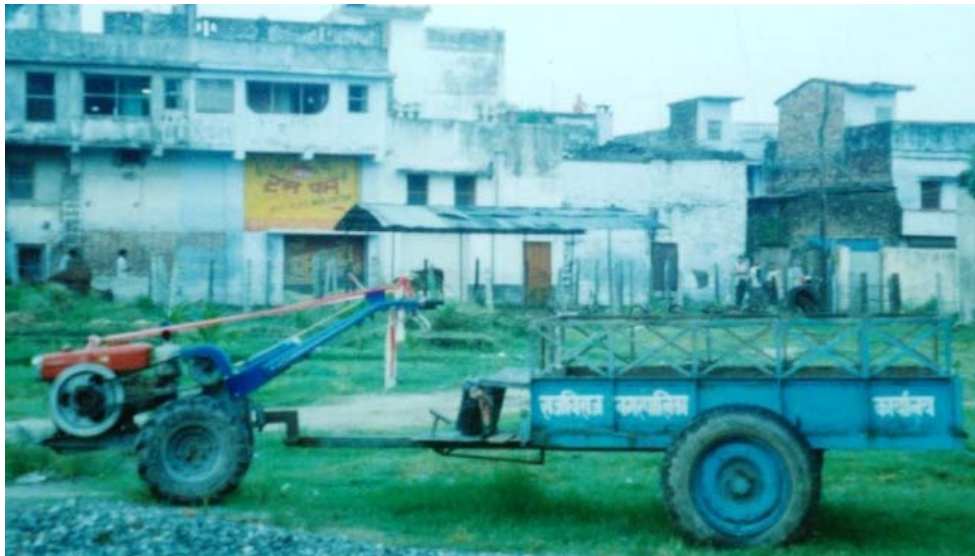
Power Tiller Used for Waste Collection
