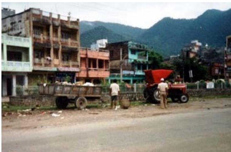
Waste Collection Using a Tractor Trailer as a Container
